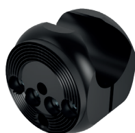
M3D RKL-T 30 11.1430 Monty 3D semi-open frame clamp for tube type Ø30 mm (1 3/16"). Apply when frame tube is not fully accessible (e.g. overlying seat). 125.00 €
